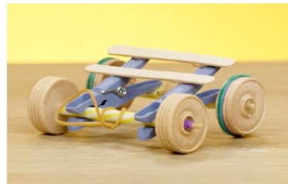
Prototype three mechanism: a rubber band is wound around the back axle and unwinds to make the car move.
