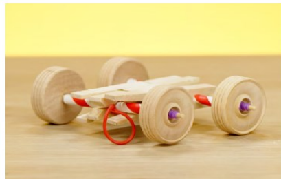
Prototype two mechanism: a rubber band is used to slingshot the car forwards.
